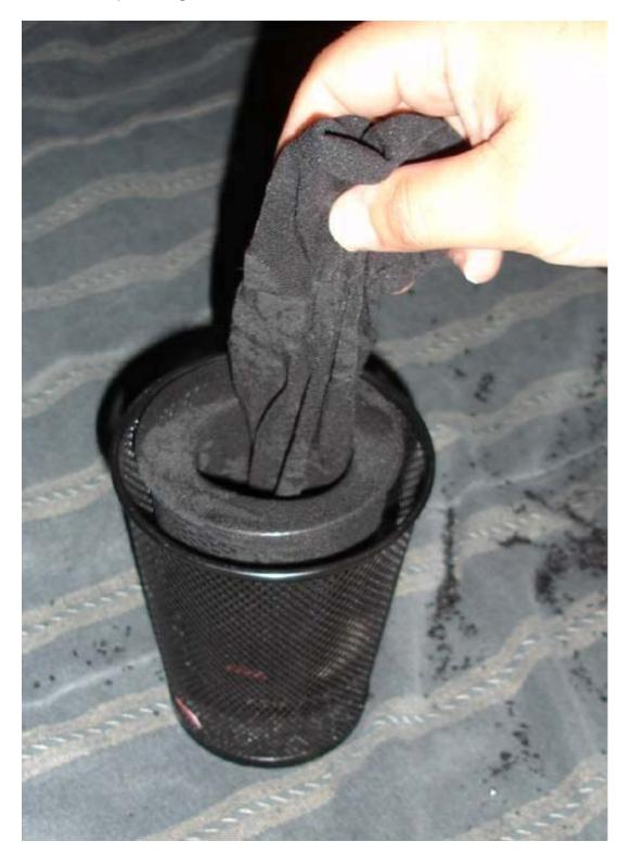
Tuck the sock into the smaller cup holding the end of the sock. Pore in the carbon.. keep holding the end of the sock.
