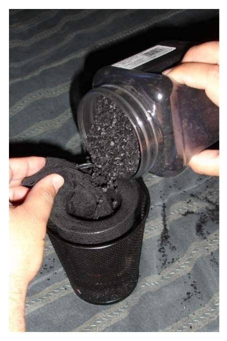
Now pull on the end of the sock and use your finger to guide the carbon into the space between both cups until filled.
